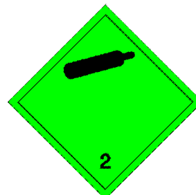
(No. 2.2) Non flammable, non-toxic gases Symbol (gas cylinder): black or white; Background: green; Figure "2" in bottom corner
